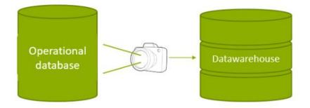
A physical datawarehouse stores data snapshots within an operational database. A logical datawarehouse however, offers transformed, user-friendly data, ready for analysis. It can disclose more data sources than only the physical datawarehouse.
