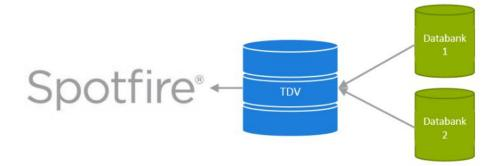
The TIBCO Data Virtualization (TDV) creates a virtual database based on (several) underlying real databases. It is a logical datawarehouse easy to use and combine data from different sources, and with an extra layer to limit access to sensitive data.
